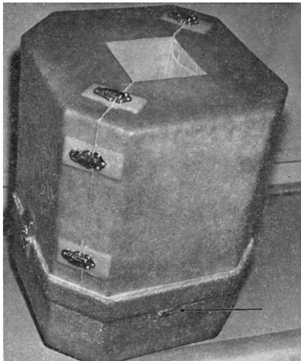
Fig. 1. Side and top view of assembled apparatus. Arrow indicates thermocouple receptacle for attachment to temperature recorder.
